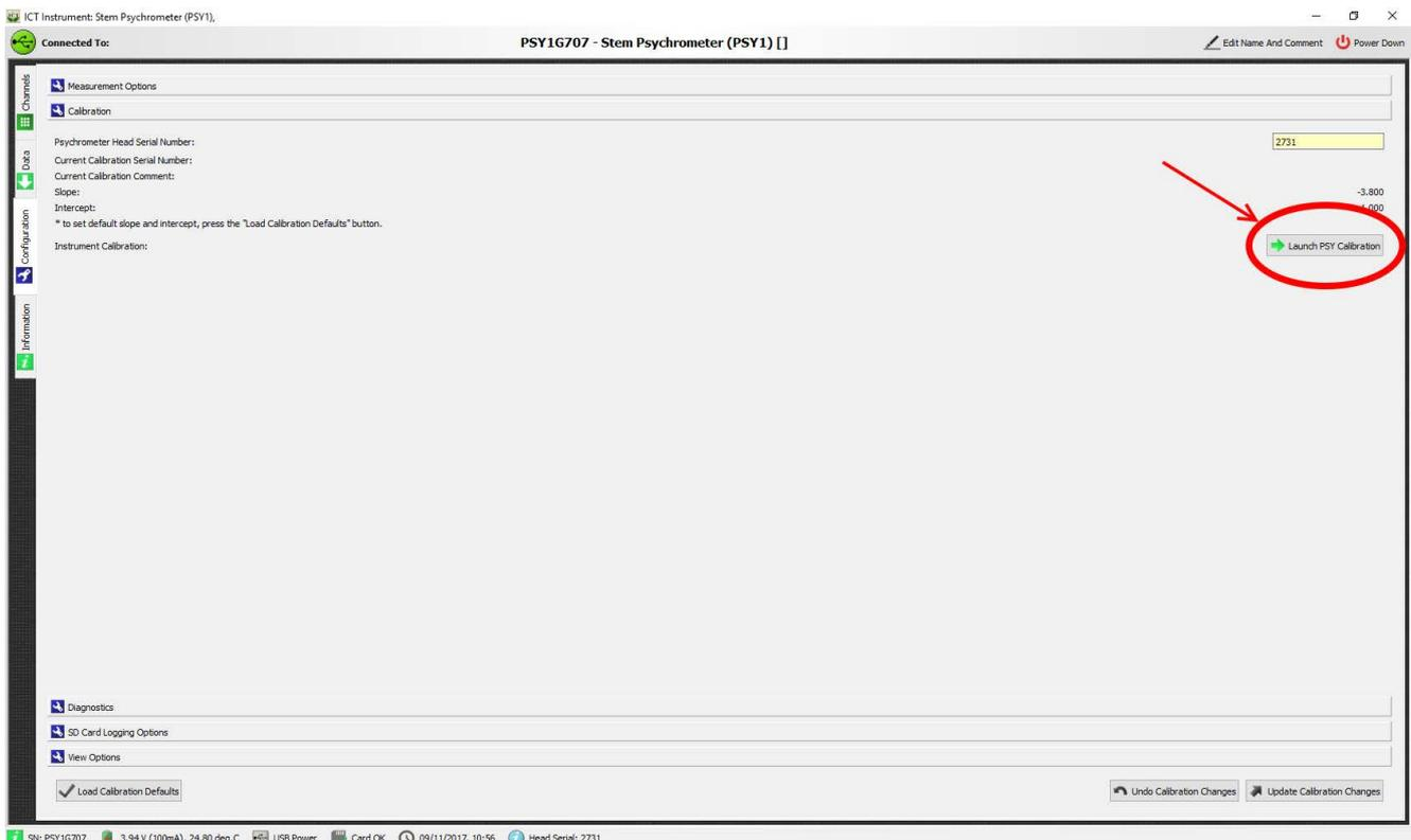
**Note:** A calibration can only be performed in Manual mode. If you attempt to “Start a Calibration” while in Live Mode or while the instrument is logging, an error message is displayed.
