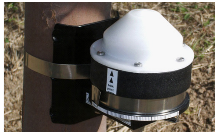
Figure 1. The DRL26 is an example stem dendrometer sensor. It can measure tree trunks with a stem diameter greater than 8cm. The DEX or LVDT dendrometers can measure smaller plant stems as well as fruits.
