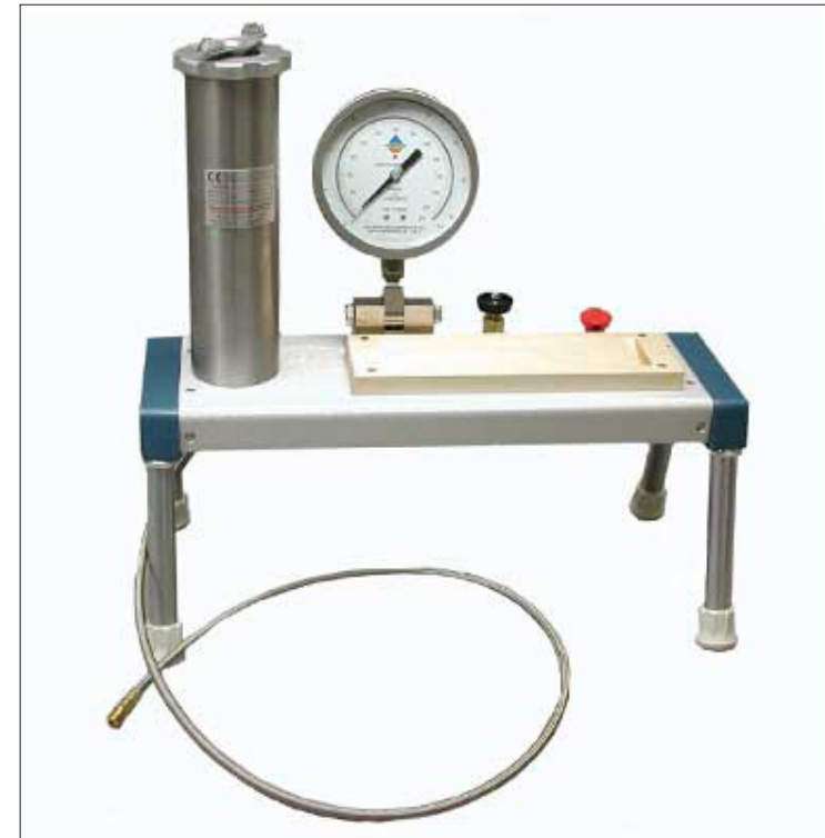
Figure 3. A plant water status console, also known as a Scholander pressure chamber or Scholander pressure bomb, has traditionally been used to measure leaf water potential.
