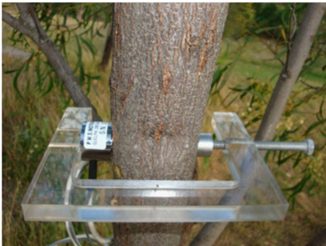
Figure 5. The PSY1 Stem Psychrometer and the sensor installed on a tree stem.
