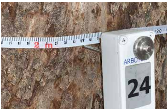
Figure 5. A tape measure around the stem cross-section allows to measure the position of each sensor easily with an accuracy of \pm 1\text{cm} ( \pm 0.4'' ).
